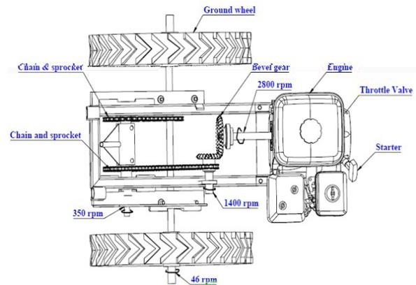
Figure 1: Diagram showing the power transmission system
