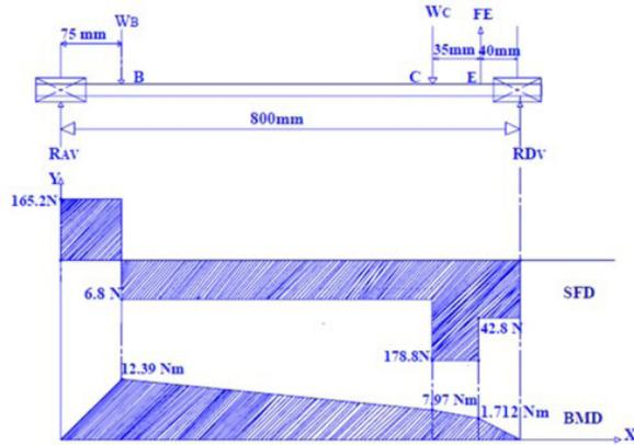
**Figure 7:** Shear forces and vertical bending moment diagrams
