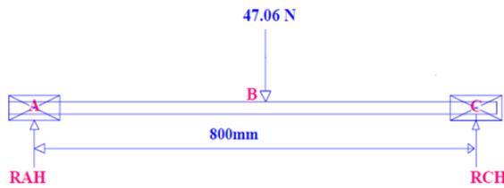
**Figure 7.1:** The reaction forces distribution on the horizontal plane
