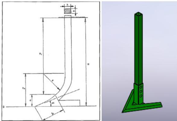
**Figure 3:** Schematic of diagram designed shank of the weeder
