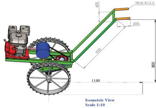
Figure 4: Diagram showing the dimensions, in mm, of the handle
