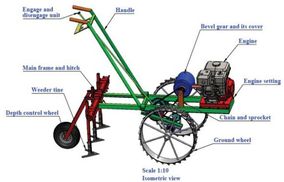
**Figure 9:** Isometric view of a designed machine
