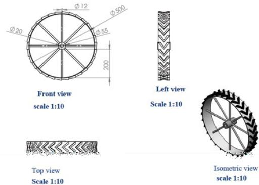
Figure 5: Details of the drive wheel
