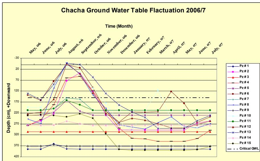
Figure 3. Water table fluctuation in the 15 piezometers
