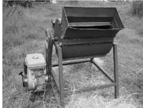
Figure 1. Developed motor driven chopper
