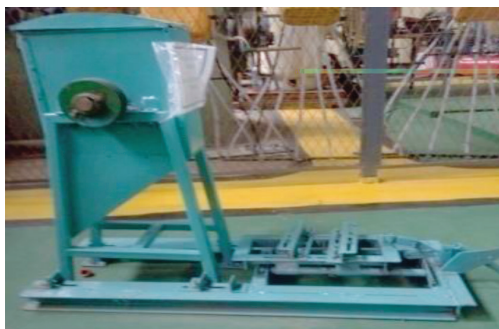
Fig 3 Newly developed engine/motor driven prototype feed chopper
