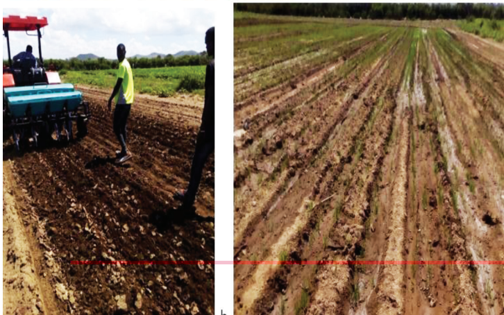
Fig. 2 A 40hp attached multi crop planter during performance evaluation.
