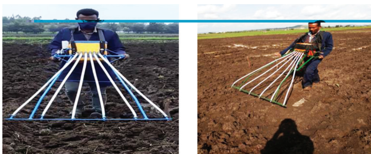
Fig.1 Front pack tef row planting machine
