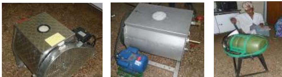
Figure 9. Milk churning devices stainless steel Electric Motor driven ELCA (left) Melkassa Electric Motor operated (middle) and Melkassa Hand Operated (right)
