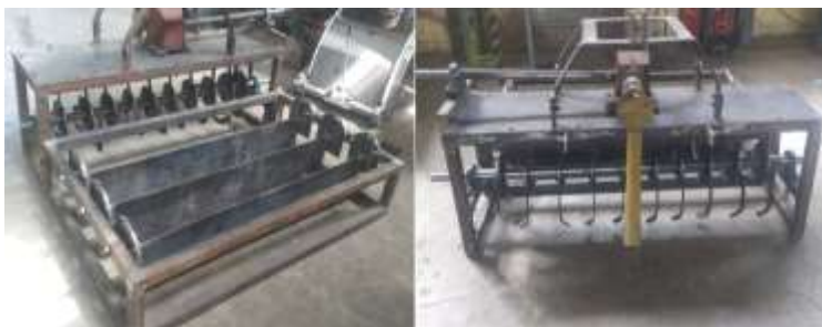
Figure 5: Newly developed small horsepower tractor attached land leveler for cereal crop
