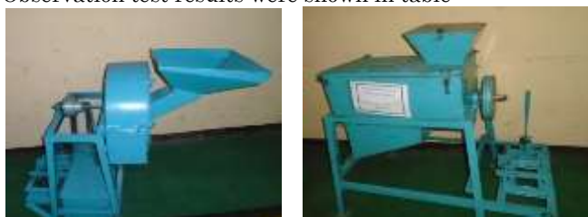
Figure4. Newly developed feed milling (left) and mixing (right) equipments
