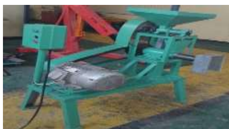
Figure 6. Existing single screw feed extruder with modified die section
