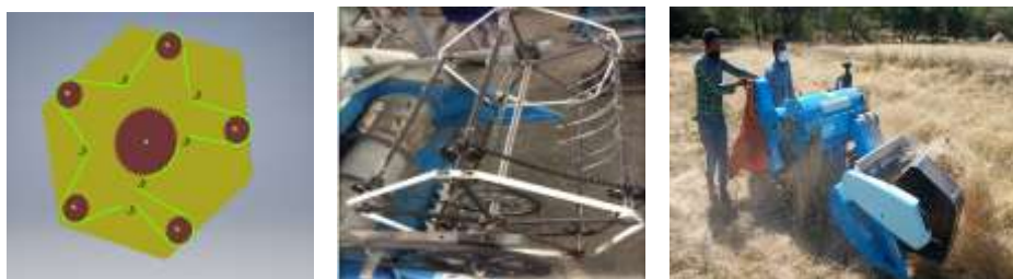
Figure 3. Developed reel mechanism and prototype mounted on mini combiner harvester
