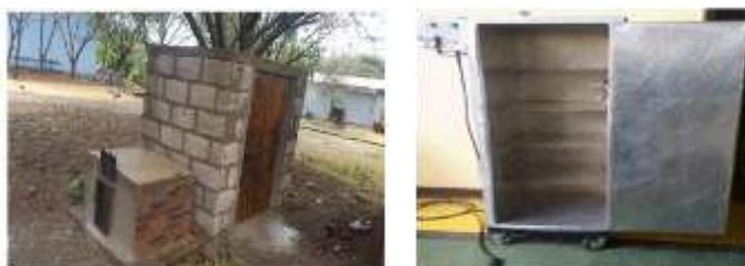
Figure 6. Stationary(left) and mobile(right) type fish smoking technology
