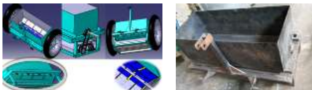
Figure 6: Newly developed small horsepower tractor attached lime spreader
