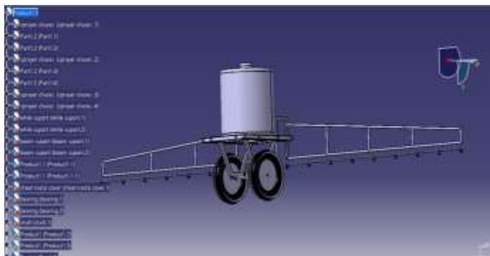
Figure 3: 3D model of two-wheel tractor attached boom sprayer
